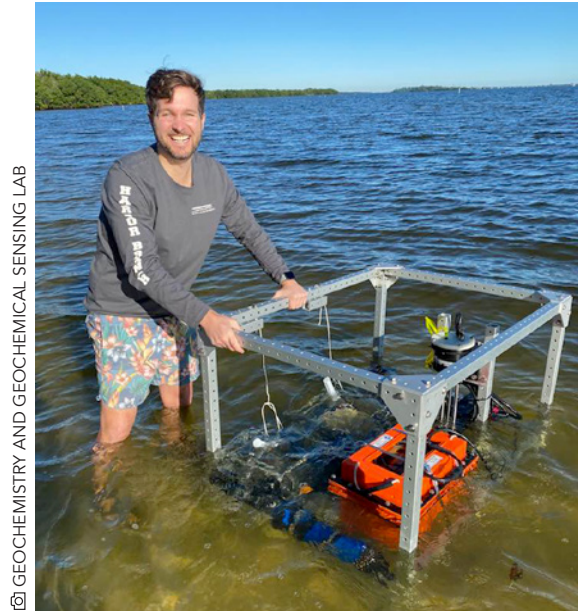
Jordon Beckler, Ph.D., tests the benthic lander in the Indian River Lagoon. The lander is capable of directly measuring the flux of nutrients from the sediments to the overlying water column.
